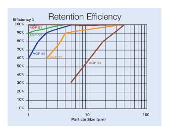
ACCUGAF Filter Bags are available in retention codes of 51, 53, 55, 57, and 59. To select the perfect ACCUGAF Filter Bag for your application use the chart and choose the retention efficiency level you need on the left side of the chart at particle size in microns at the bottom. Next find which bag efficiency code (identified by the colored lines) is closest to that point. There you have it, the most cost effective filter bag for your critical filtration application.
