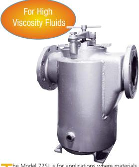
he Model 72SJ is for applications where materials must be kept hot in order to remain fluid. Examples are chocolate, asphalt, resins and polymers. The strainer body temperature is maintained by circulating steam or a heat transfer fluid through the strainer jacket.
