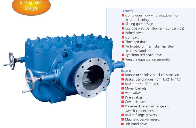
he Eaton Model 570 Duplex Basket Strainer has been specifically designed to remove potential damage causing particles from large volumes of water and other process media (up to 30,000 gpm) efficiently and cost effectively. The strainer operates continuously and the pipeline flow never has to be shut down for strainer basket cleaning.
